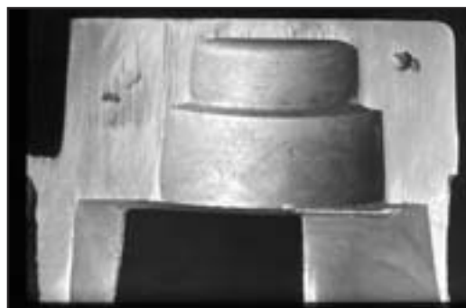
Figure 3. Shrinkage porosity - lack of feeding-casting.
