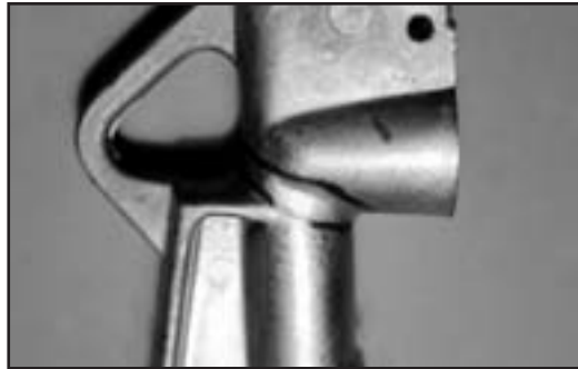
Figure 5. Hot tearing - composition, hot spots-casting.
